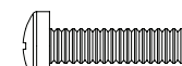
4x M6 x 25mm philips screws (F) 4 vis cruciformes M6 x 25mm (F)
