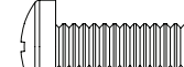
4x M8 x 25mm philips screws (H) 4 vis cruciformes M8 x 25mm (H)
